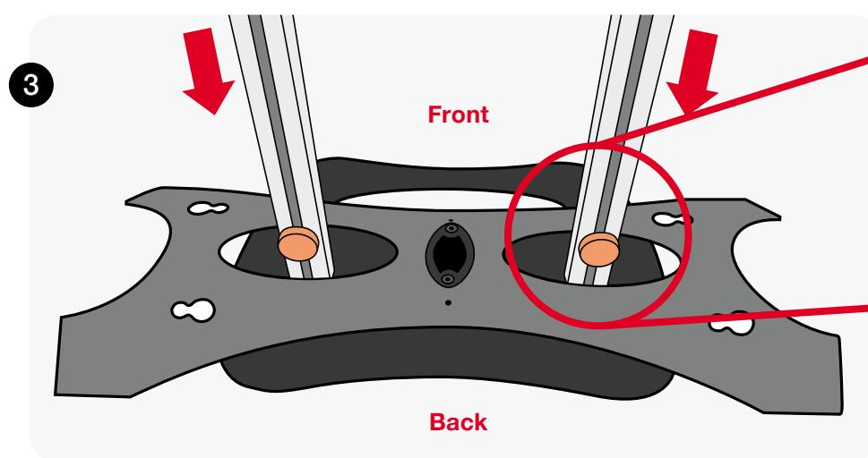
Slide the bottom AV uprights (orange fixing) on to the AV base, and tighten the orange screws.
