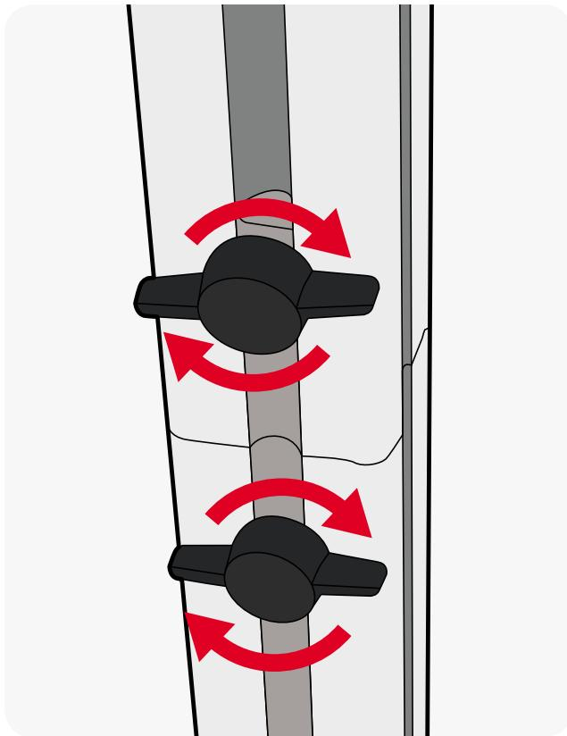
Place the next section of AV upright onto the locating pin and slide a locking pin between the joint and tighten.
