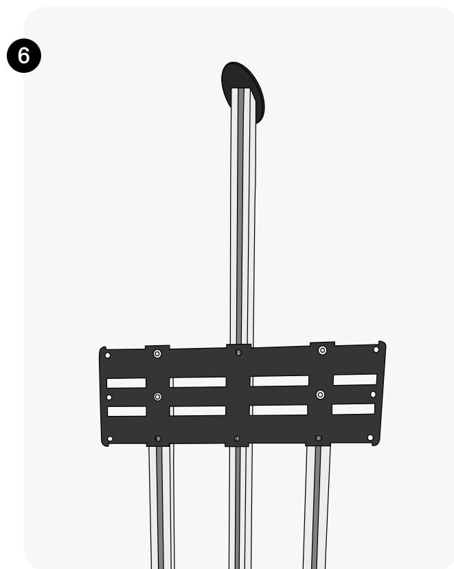
Continue to build the TWIST stand; making sure that the TWIST upright sits behind the AV crossbeam.
