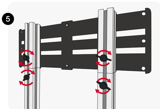
Locate the AV crossbeam into position and tighten the locking pins.
