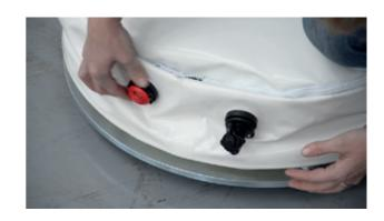
Red overpressure valves must be installed on their positions, well tighted to prevent air leak.
