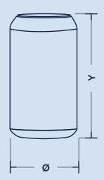
AXION Inflatable Can has the same principle as the AXION Tube, but is patterned in a can shape. It is a sealed inflatable with an internal bladder and higher internal pressure than traditional inflatable cans. It has better weather resistance, better stability and no blower noise.
