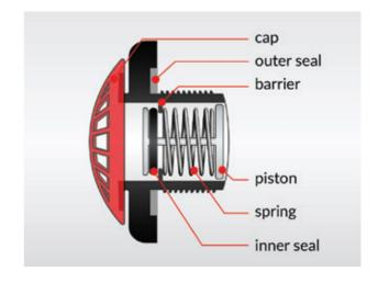
In a case arch was not used for longer time period, it is recommended to check functioning of all overpressure valves by pushing the spring with a finger or blowing through the valve. Parallelly, seats of all valves shall be checked to avoid sand grains or dirt to block closing the valve.
