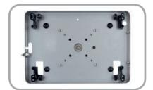
4. Position holes of iPad Air inserts over locating pins and gently push-fit into enclosure.
