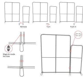
Remove one foot from second frame and align both frames on one foot
